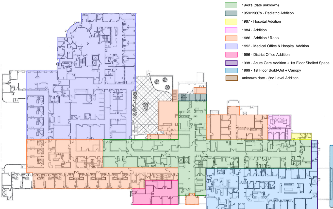
Level 1 Year of Construction Floor Plan
