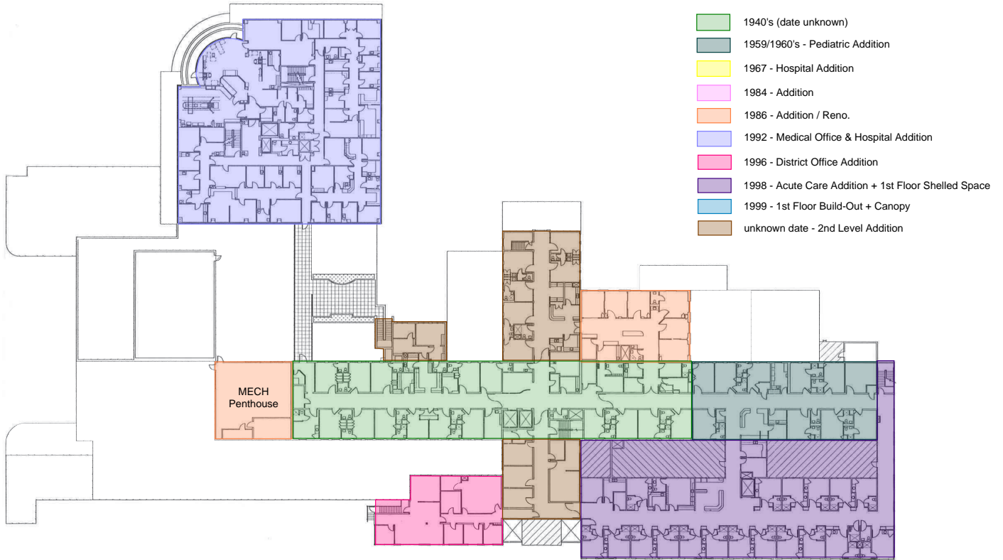
Level 2 Year of Construction Floor Plan
